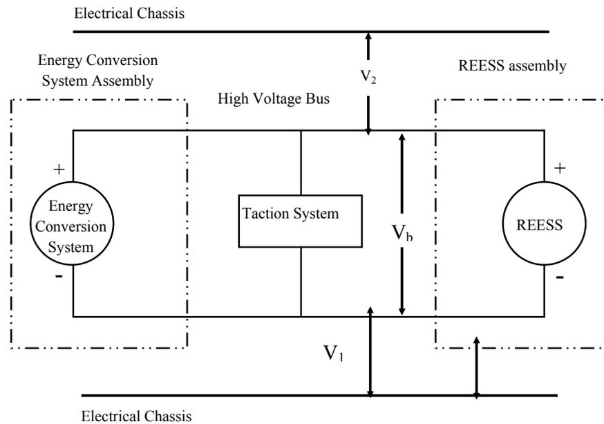
Figure 1 Measurement of  $V_b$ ,  $V_1$ ,  $V_2$
